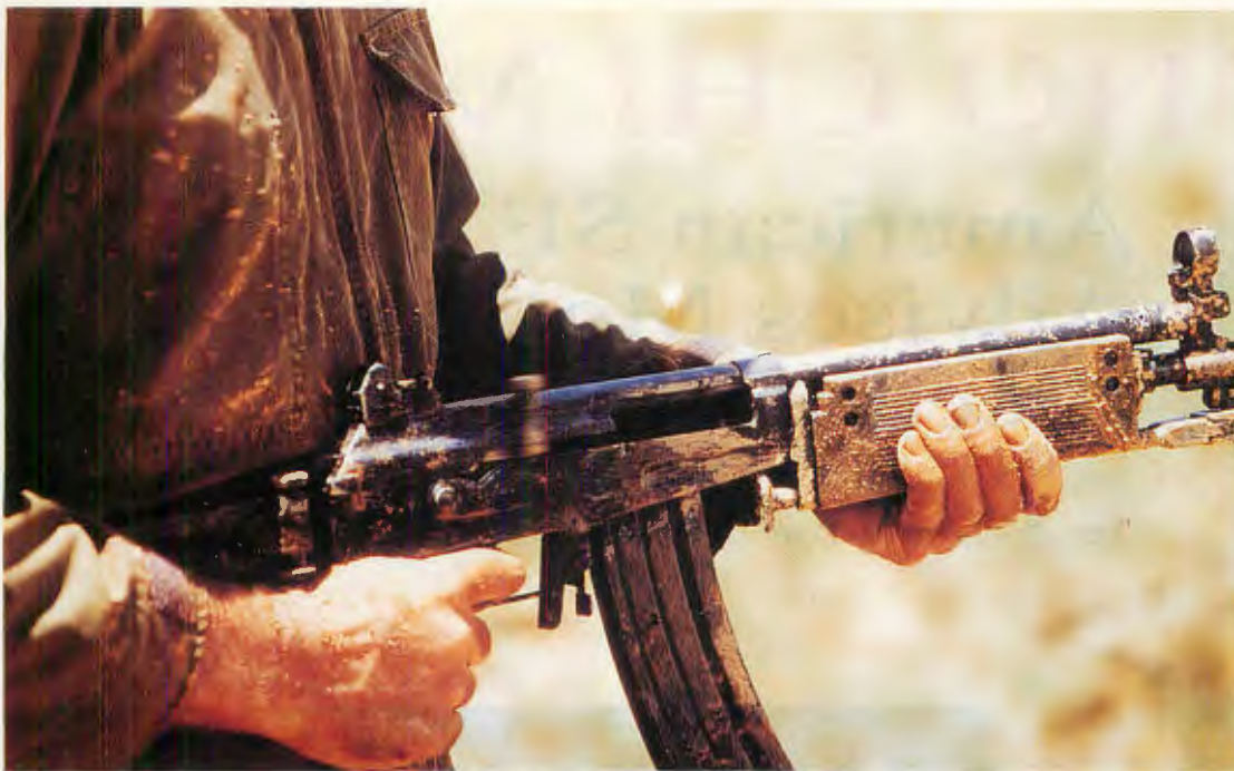
Without doubt the most unusual transmutation of an infantry rifle in the history of military small arms, the Vektor H5 is a commercial, slide-action version of the gas-operated, selective-fire R4. Photo: courtesy LIW
